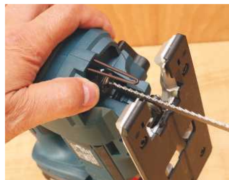
▲ Slide the collar around and the blade is ejected without having to touch it
